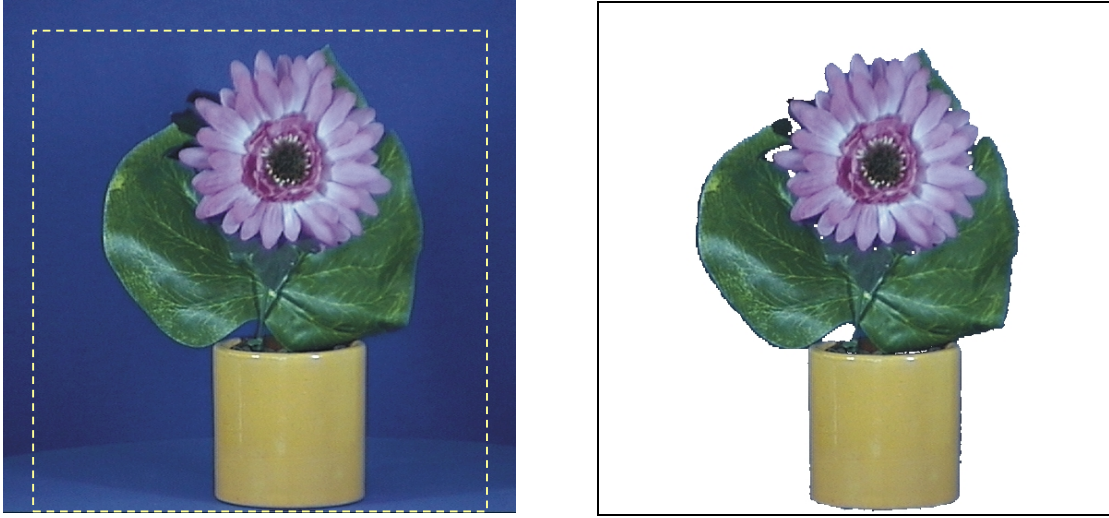
Figure 3: Background estimation using an IHS color space histogram (left) and the resulting silhouette extraction (right).
