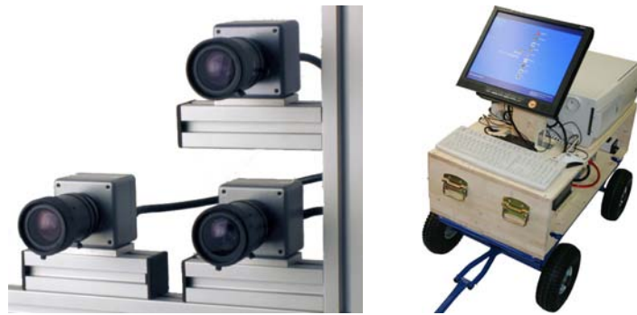
Fig. 1: a) Trinocular stereo rig with mounted Scorpion cameras and b) the mobile image acquisition system.
