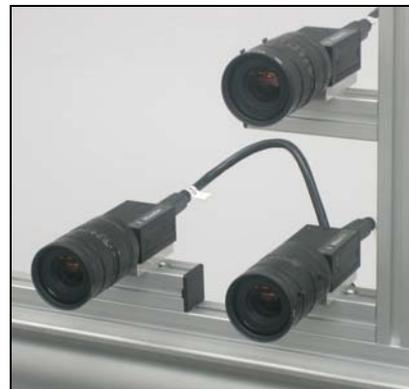
Figure 1. Mobile trifocal camera system
