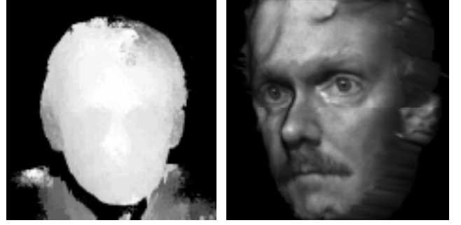
Fig. 3: Enhanced depth map using hierarchical Block Matching and the 3-D reconstruction with texture mapping.
