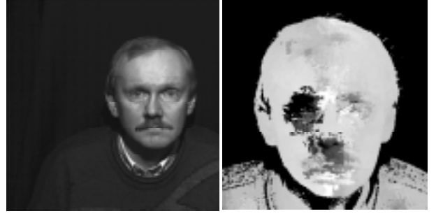
Fig. 1: Gray value reproduction of the left color stereo image "ANDREAS" and the depth map (right) obtained when applying standard Block Matching to the images.
