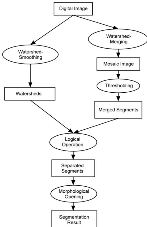
**Figure 7:** Overview of the combined watershed algorithm
