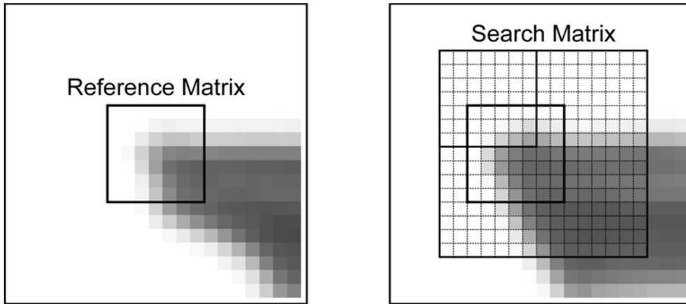
**Figure 1:** Classical matching approach, as used for measurement of tie points
