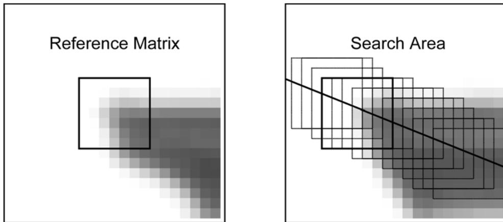
**Figure 3:** Matching along the epipolar line in the restitution process
