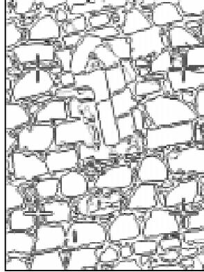
**Fig. 3b:** Result of an edge detection (*black*) followed by a contour tracing (*gray*)
