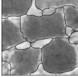
**Fig. 6b:** Shifted contours of the watershed transform using a smoothed gradient
