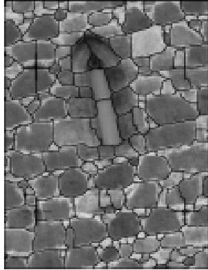
**Fig. 8a:** Separation of stones using the watershed transform on a smoothed gradient
