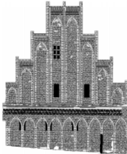
**Fig. 1b:** CAD-Model of the analytical measured facade
