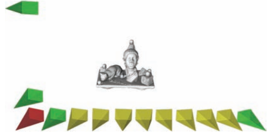
Figure 5: Orientation of the reference image (red), narrow- and wide-baseline stereo images (green) and the linear motion sequence (yellow)
