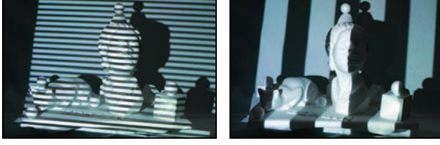
Figure 14: Examples of binary coded textures (9 images with horizontal and 10 images with vertical stripes)
